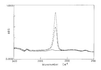
**Figure 1** FTIR of ungrafted PP fiber (—) and PP-*g*-PAN fibers containing (-.-.) 7% and (--.) 11% graft.
