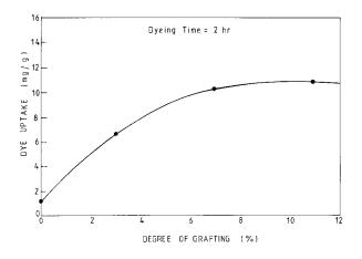
**Figure 4** Variation of the dye uptake with the degree of grafting in PP-g-PAN fibers.
