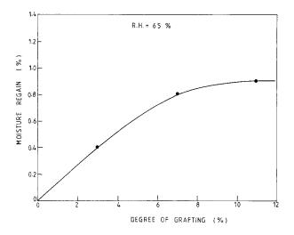
**Figure 2** Variation of the moisture regain with the degree of grafting in PP-g-PAN fibers.
