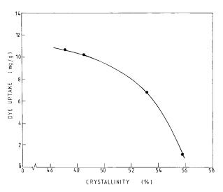
**Figure 5** Variation of the dye uptake with the crystallinity in PP-g-PAN fibers.
